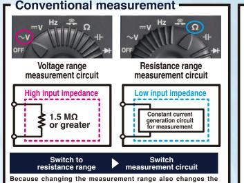
Because changing the measurement range also changes the measurement circuit, mistakenly inputting voltage with the instrument set to the resistance range will cause a large current to flow to the device, leading to hazards such as tripped circuit breakers and arcing.
