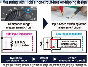
The measurement circuit is switched after the instrument detects resistance, continuity, capacitance, or diode input. Even if you mistakenly input voltage with the instrument set to the resistance range, the high input impedance will limit the current flowing to the instrument to 1.5 mA or less to prevent potential hazards.
